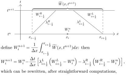
$$W_i^{n+1} = W_i^n - \frac{\Delta t}{\Delta x} \left( \mathcal{F}_{i+\frac{1}{2}}^n - \mathcal{F}_{i-\frac{1}{2}}^n \right) + \Delta t \left( \begin{pmatrix} 0 \\ (\mathcal{S}_{\text{topo}})_i^n \end{pmatrix} + \begin{pmatrix} 0 \\ (\mathcal{S}_{\text{fric}})_i^n \end{pmatrix}_{1 \not {b} / 26} \right)$$
