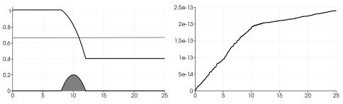
left: initial free surface and free surface for the steady state solution, obtained after a transient state right: error on the discharge
