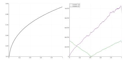
small perturbation of a steady state solution left: water height; right: errors to the equilibrium
