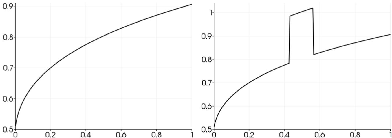
left panel: water height for the subcritical steady state solution
