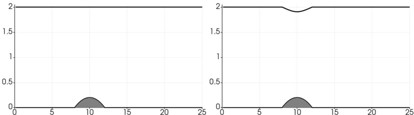
left panel: initial free surface at rest; water is injected from the left boundary
