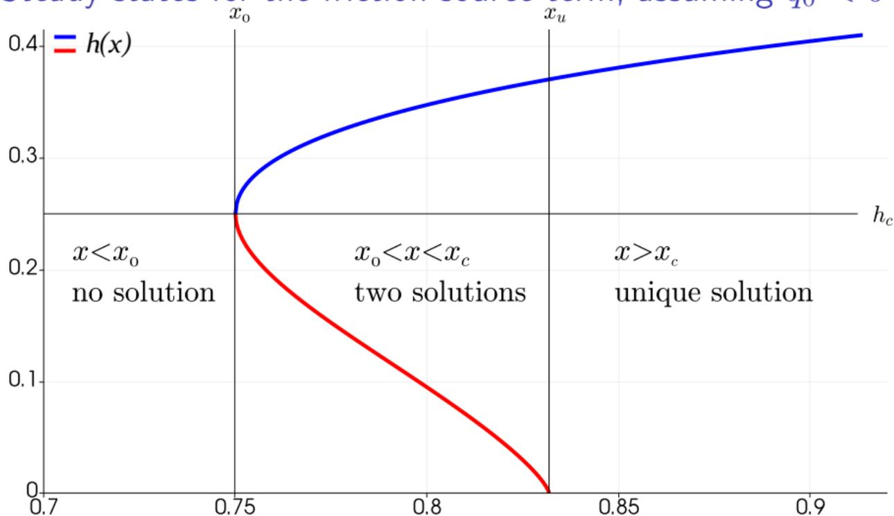
blue curve: subcritical solution; red curve: supercritical
