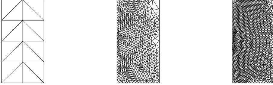
Figure 10: Third example. Initial (left) and refined meshes in adaptive procedure
