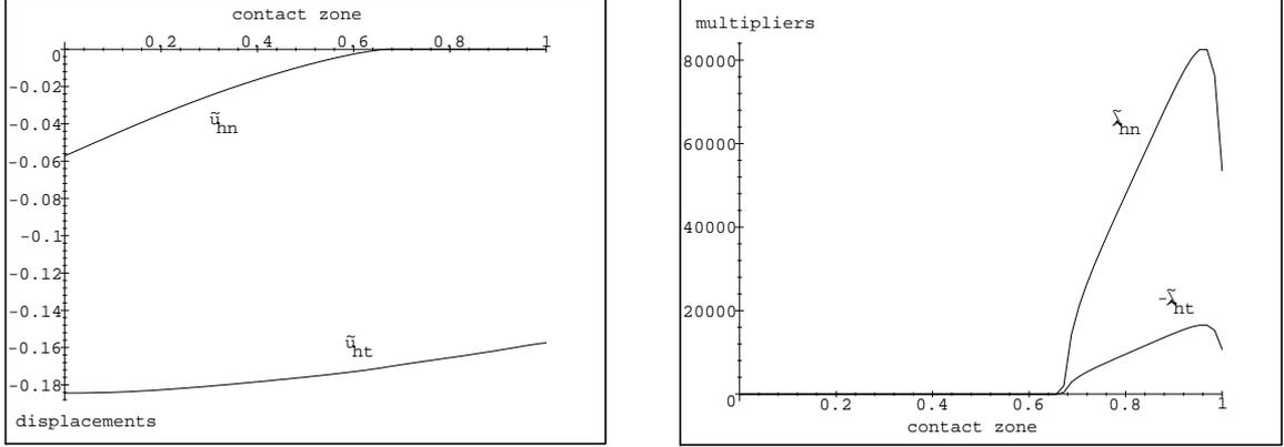
Figure 2: First example. Left: normal and tangential displacements ( $\tilde{u}_{hn}, \tilde{u}_{ht}$ ) on  $\Gamma_C$ . Right: normal and tangential multipliers ( $\tilde{\lambda}_{hn}, -\tilde{\lambda}_{ht}$ ) on  $\Gamma_C$ .
