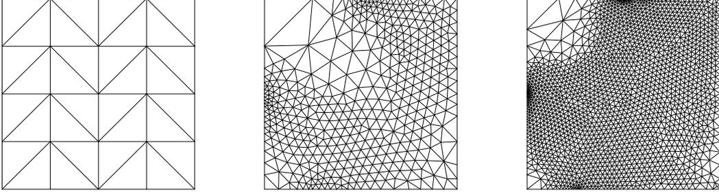
Figure 6: Second example. Initial (left) and refined meshes in adaptive procedure
