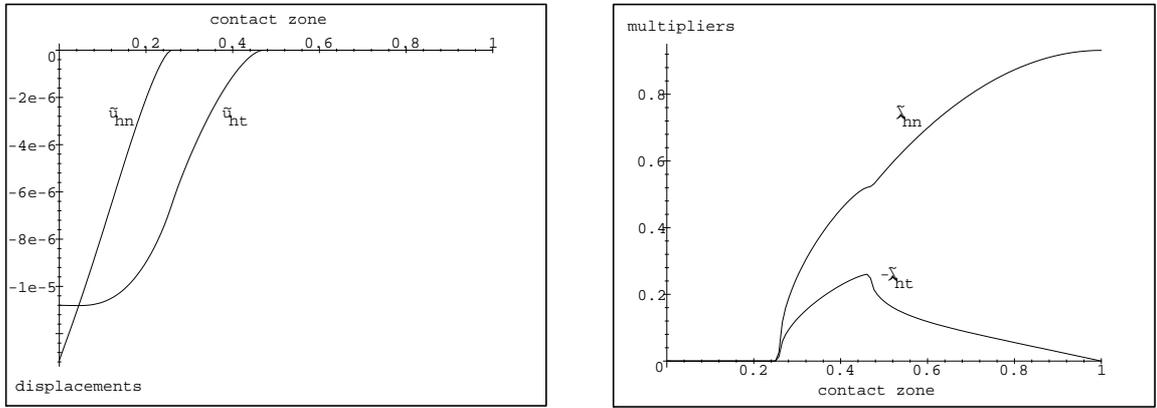
Figure 5: Second example. Left: normal and tangential displacements  $(\tilde{u}_{hn}, \tilde{u}_{ht})$  on  $\Gamma_C$ . Right: normal and tangential multipliers  $(\tilde{\lambda}_{hn}, -\tilde{\lambda}_{ht})$  on  $\Gamma_C$ .
