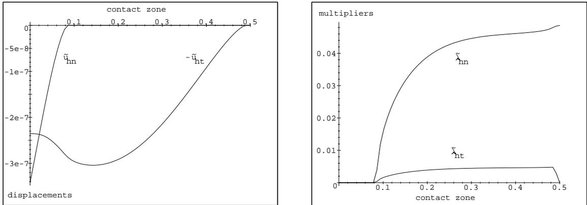
Figure 9: Third example. Left: normal and tangential displacements  $(\tilde{u}_{hn}, -\tilde{u}_{ht})$  on  $\Gamma_C$ . Right: normal and tangential multipliers  $(\tilde{\lambda}_{hn}, \tilde{\lambda}_{ht})$  on  $\Gamma_C$ .
