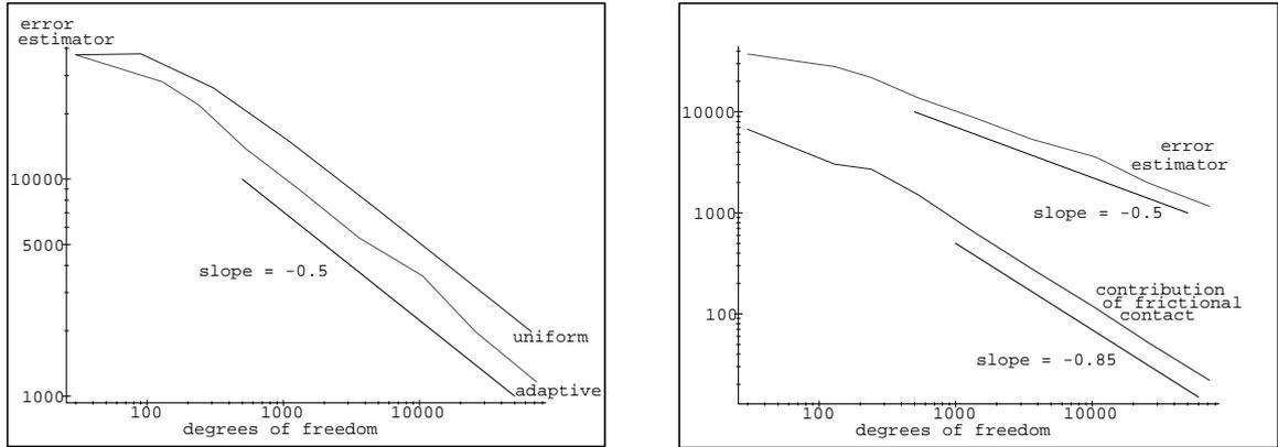
Figure 11: Third example. Left: Convergence of the error estimator  $\tilde{\eta}$  with uniform and adaptive refinement. Right: Convergence of the error estimator  $\tilde{\eta}$  and its frictional contact contribution  $\tilde{\eta}_C$  with adaptive refinement.
