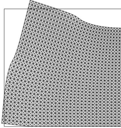
Figure 4: Second example. Initial and deformed configurations with  $\mu = 0.5$  and  $N_C = 32$  (deformation is amplified by a factor 2000).
