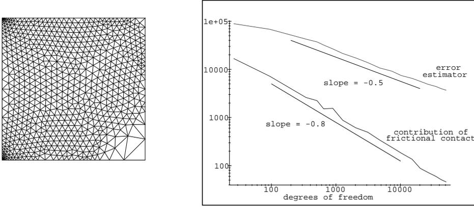
Figure 3: First example. Left: Adapted mesh. Right: Convergence of the error estimator  $\tilde{\eta}$  and its frictional contact contribution  $\tilde{\eta}_C$  with adaptive refinement.
