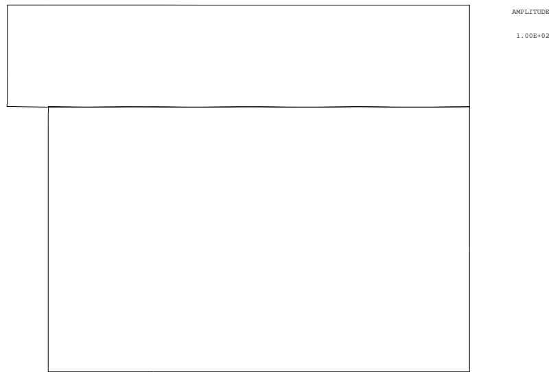
Figure 13: Deformed configuration with the symmetrical definition of local contact (amplification: 100)
