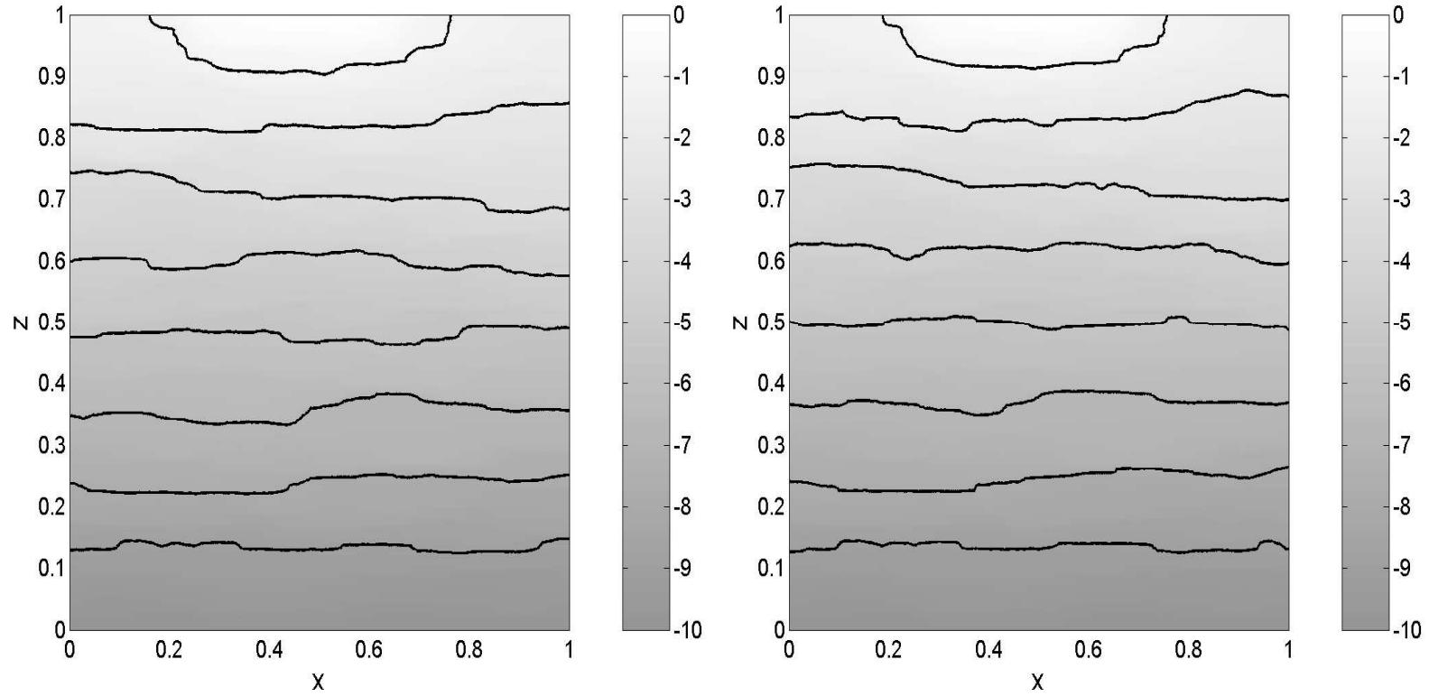
Exponential model with anisotropic heterogeneity. Comparison of water pressure between the fine model (left) and the coarse model (right).
