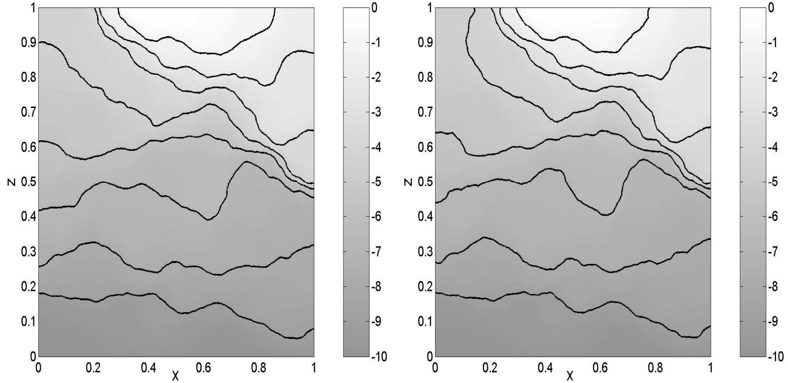
Exponential model with isotropic heterogeneity. Comparison of water pressure between the fine model (left) and the coarse model (right).
