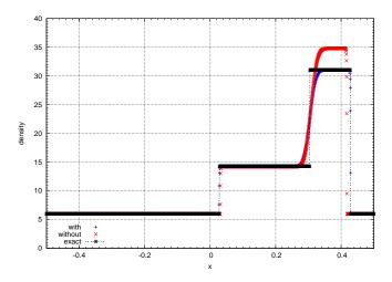
Riemann problem - Results obtained with and without corrective terms in the internal energy balance.
