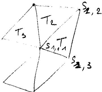
$$V_h = \left\{ v \in C([0,1]) ; v \Big|_{T_i} \in \underbrace{R^1[x,y]}_{ax + by + c} \right\}$$
