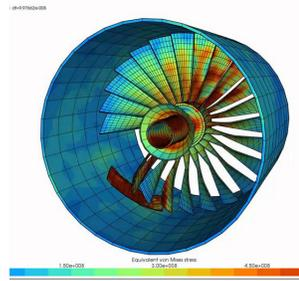
(L) A FE mesh in Earth Sciences. (M) A FE analysis of an aircraft engine: Von Mises stress values. (R) Model reduction
