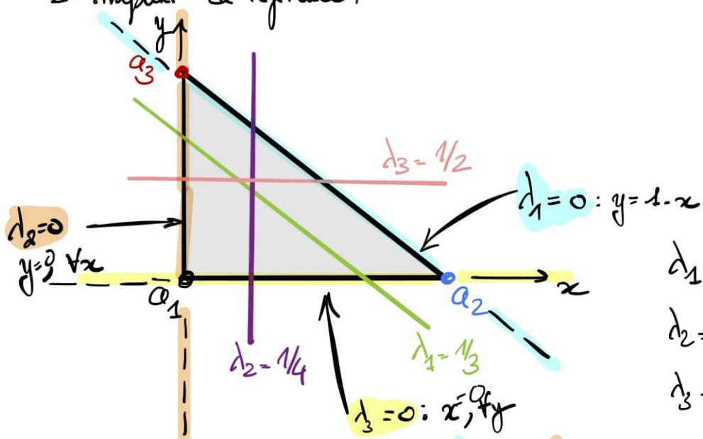
$$\begin{aligned}d_1(x,y) &= 1-x-y \\d_2(x,y) &= x \\d_3(x,y) &= y\end{aligned}$$
