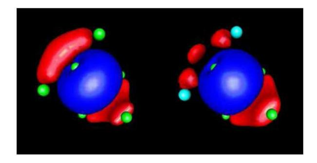
Amplitude **isosurface contours** for maximally-localized Wannier functions in **Si** (left panel) and **GaAs** (right panel). Red and blue contours are for isosurfaces of identical absolute value but opposite signs; Si and As atoms are in green, Ga in cyan. Notice that **breaking of inversion symmetry** in GaAs polarizes the WFs towards the more electronegative As anion.
