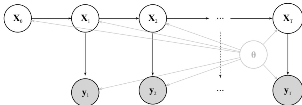
Figure : Graph representation of a general HMM.
