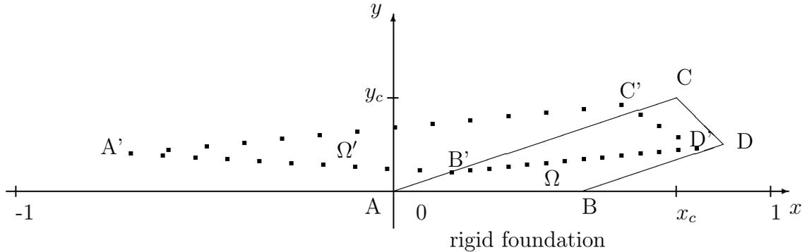
Figure 5: Initial configuration  $\Omega = ABDC$  (solid line) and the first deformed configuration corresponding to separation  $\Omega' = A'B'D'C'$  (dotted line). The second deformed configuration corresponding to stick is  $\Omega'' = ABD'C'$ .
