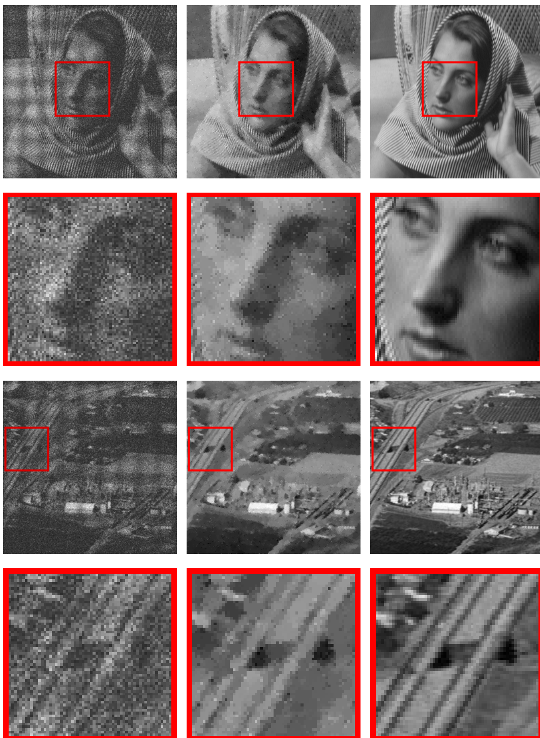
Figure 9: Reconstruction of the images “barbara” (first and second rows) and “factory” (third and fourth rows) with a noise level \sigma = 0.1 . The remaining parameters are set as follows: \bar{w} = 16.2 , \sigma_c = 0.81 and \sigma_w = 0.07 . The left column correspond to partial available data where each pixel is assigned its maximum intensity over all k \in \{1, \dots, K\} . The middle and right columns correspond resp. to the image estimate and the ideal image. Detailed views of all these images are also provided on the second and fourth rows.
