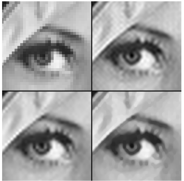
Figure 3: Up-left : Part of Lenna image zoomed x8 by duplication. Up-Right : Zoom by the zero-padding method. Down-left : Zoom yields by the minimisation of the H^1 semi-norm. Down-right : Zoom yields by the minimisation of the total variation of the image.
