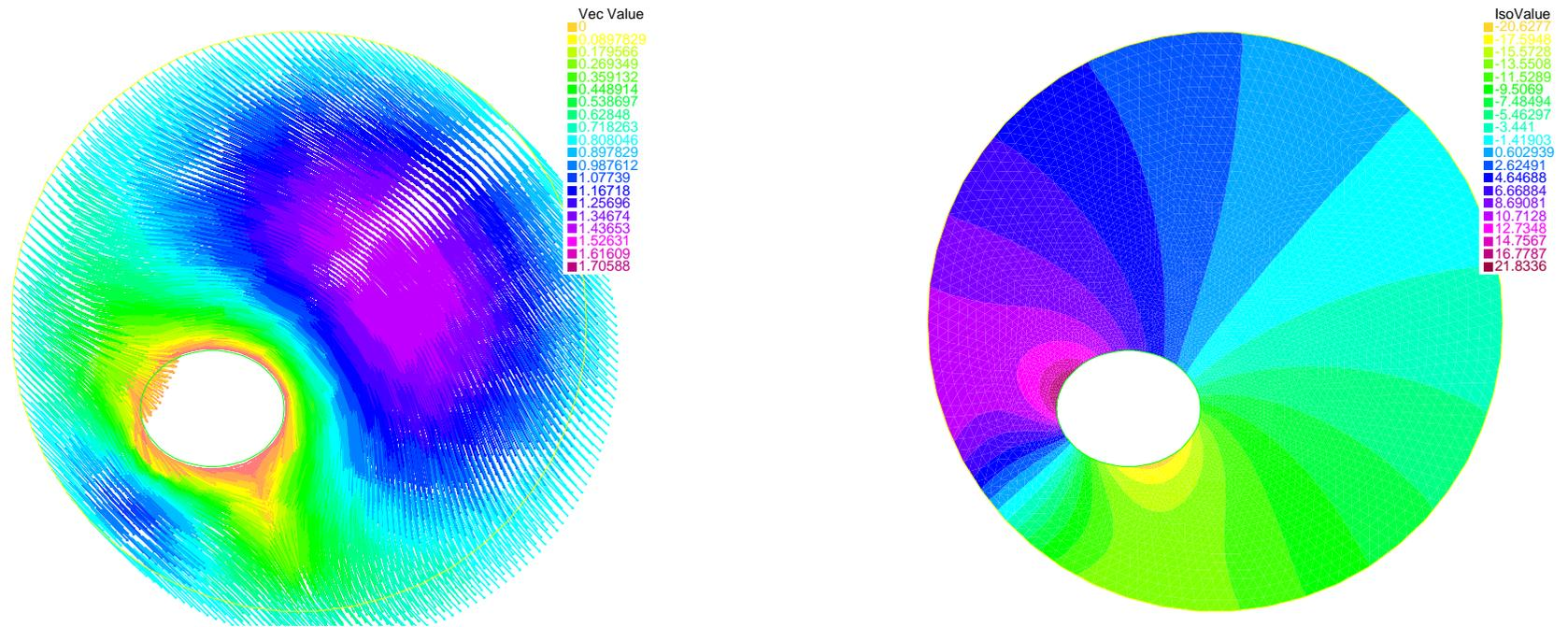
First obstacle : velocity field and pressure field
