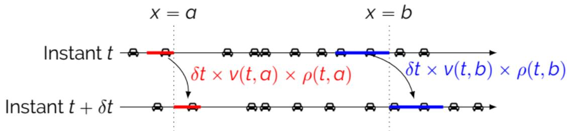
$$\int_a^b \frac{\rho(t + \delta t, x) - \rho(t, x)}{\delta t} dx = - \int_a^b \frac{\partial}{\partial x} (\rho(t, x) v(t, x)) dx.$$
