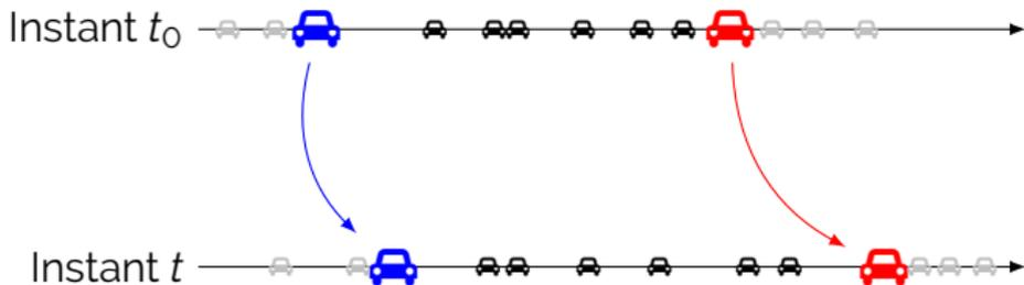
$$0 = \left( \frac{d}{dt} X(t, \text{red car}) \right) \rho(t, X(t, \text{red car})) - \left( \frac{d}{dt} X(t, \text{blue car}) \right) \rho(t, X(t, \text{blue car})) \\ + \int_{X(t, \text{blue car})}^{X(t, \text{red car})} \frac{\partial \rho}{\partial t}(t, x) dx.$$
