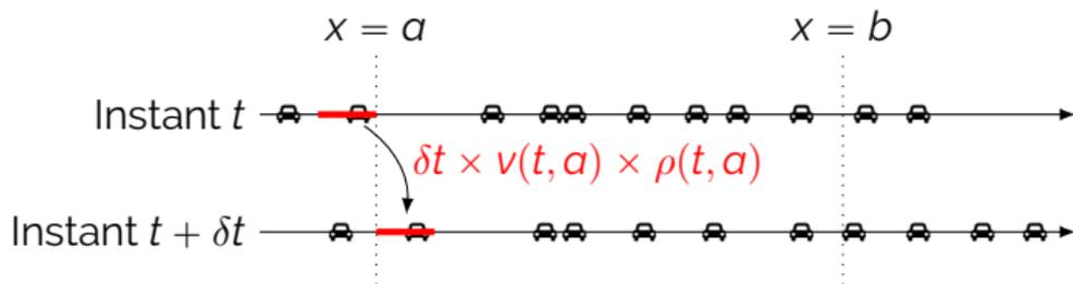
$$\int_a^b \rho(t + \delta t, x) dx - \int_a^b \rho(t, x) dx = (\delta t)v(t, a)\rho(t, a) - \text{véh. sortants}$$
