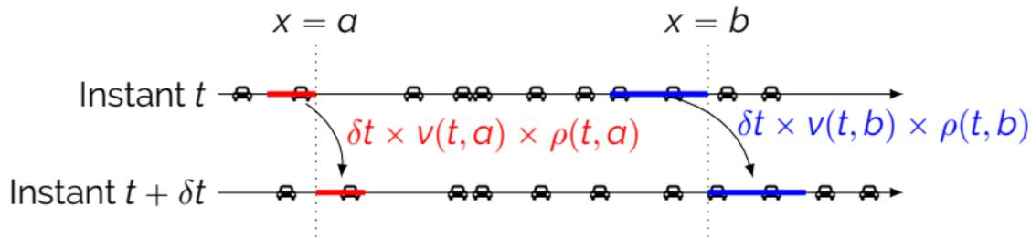
$$\delta t \text{ petit} \implies \int_a^b \left( \frac{\partial \rho}{\partial t} + \frac{\partial(\rho v)}{\partial x} \right) (t, x) dx = 0.$$
