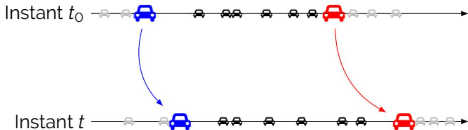
$$0 = \int_{x(t, \text{blue car})}^{x(t, \text{red car})} \left( \frac{\partial \rho}{\partial t} + \frac{\partial}{\partial x}(\rho v) \right) dx.$$
