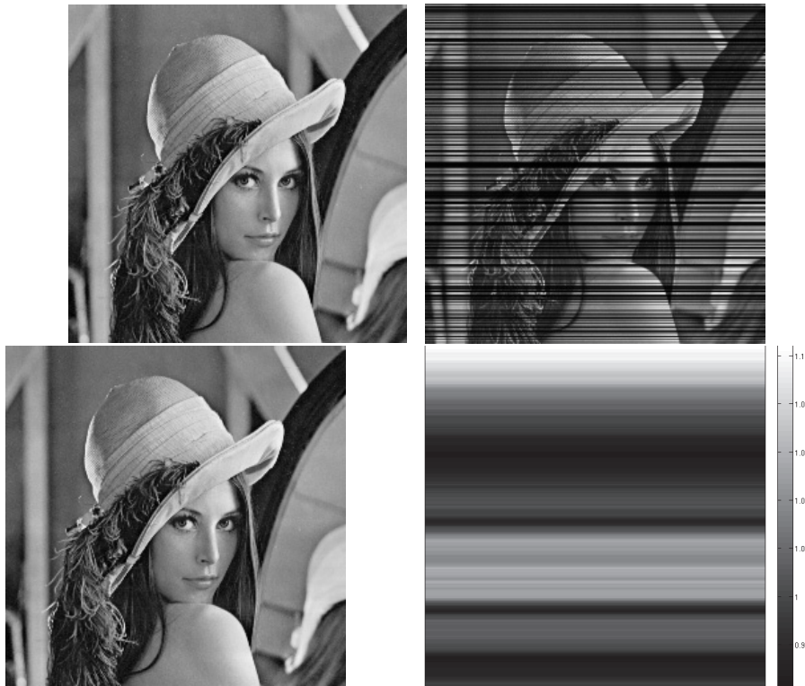
Figure 3. An example involving a multiplicative noise model. Top-left: original image. Top-right: noisy image. It is obtained by multiplying each line of the original image by a uniform random variable in [0.1, 1] . SNR=10.6dB – Bottom-left: denoised using the method proposed in [9] on the logarithm of the noisy image. SNR=29.1dB – Bottom-right: ratio between the original image and the denoised image. The multiplicative factor is retrieved accurately.
