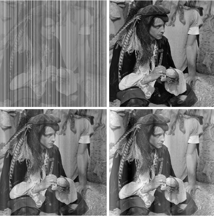
Fig. 5. Top-left: noisy pirate. Top-right: denoised using VSNR. Bottom-left: denoised using DeStripe [7]. Bottom-right: denoised using Wavelet-FFT [16]. This experiment corresponds to the last line of Table I. The noise pattern is a vertical line. The DeStripe and Wavelet-FFT algorithms do not completely remove low frequencies while VSNR leads to near perfect results.
