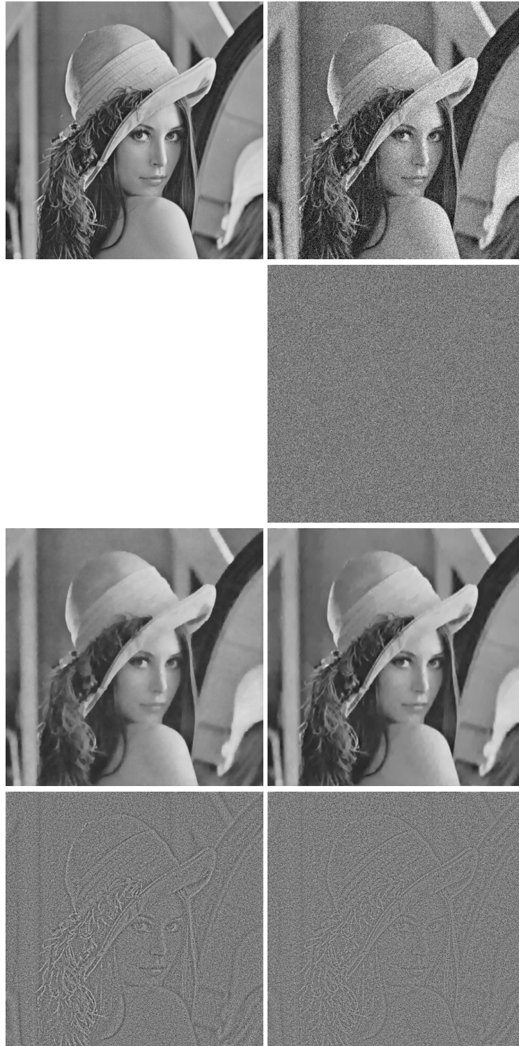
Fig. 5. Denoising results for a true example. First row, from left to right: original image, noisy image (SNR=15.4dB), denoised with TV and a regularization parameter maximizing the SNR (SNR=23.1dB, worst z -score: 69.9), denoised with the bilevel approach (SNR=24.5dB, worst z -score: 7.7). Second row: residuals associated to the top images. (same scale for the gray-level).
