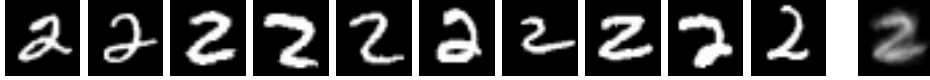
Figure 3.4: Naive mean (right image) of a set of 10 images (mnist database, 28 \times 28 pixels images, see [LBBH98] for more details on this data set).
