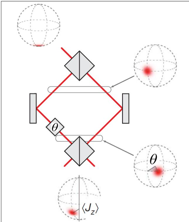
Interferometer = **ROTATION OF THE INPUT STATE**
