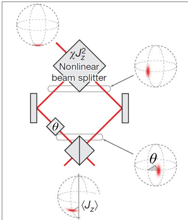
Interferometer = **ROTATION OF THE INPUT STATE**
